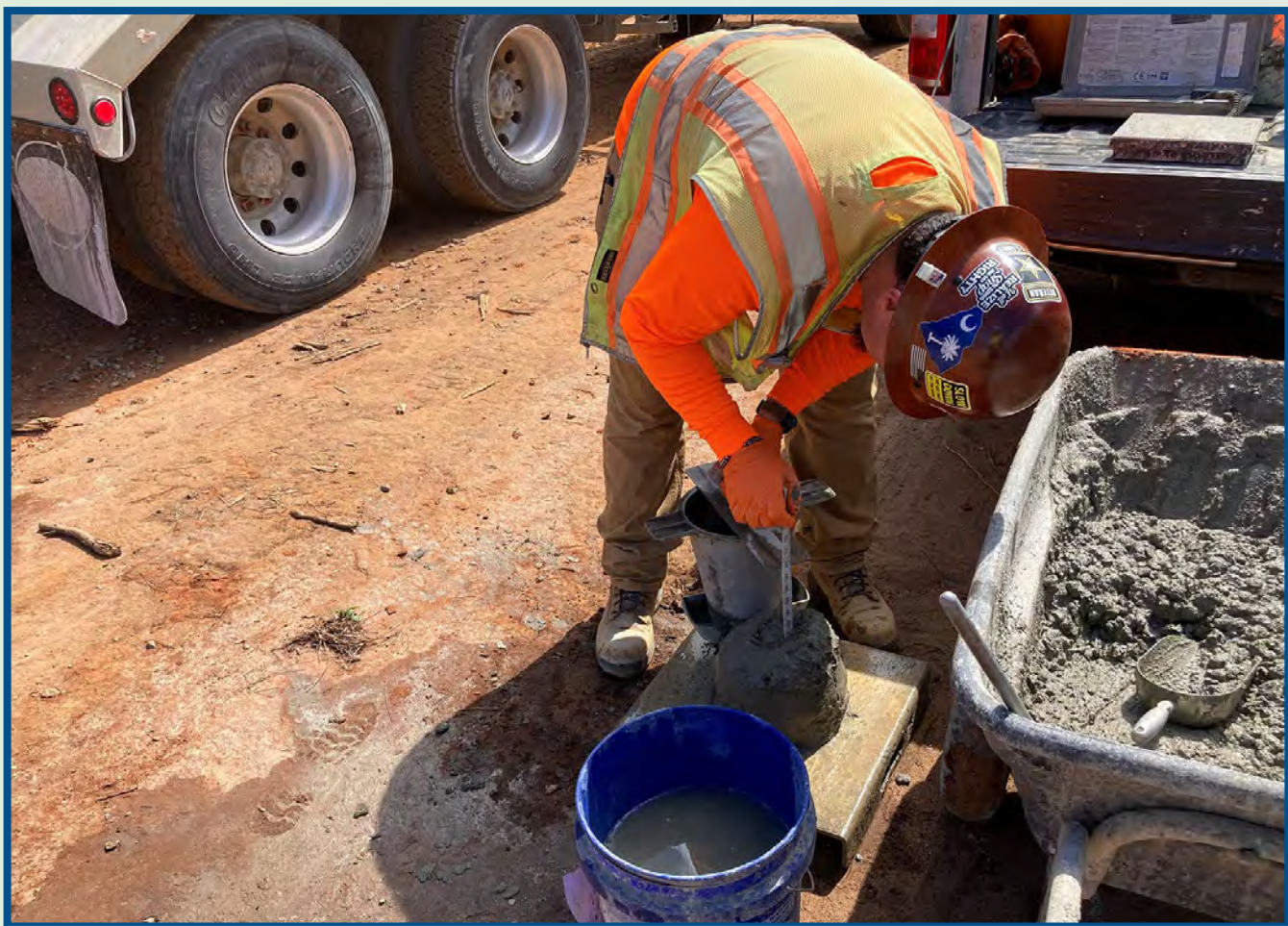
Concrete technician performing field slump test on concrete, February 2024
